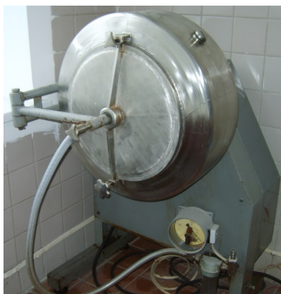
Fig. 1 – Laboratory setup for wet salting of meat raw materials Ya5-FMS
