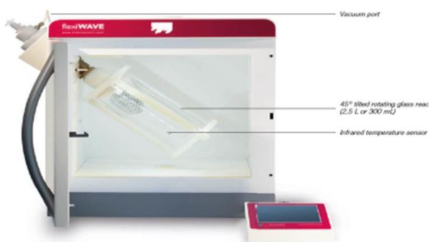
Figure 2 – Microwave laboratory rotary reactor for solid-phase reactions, including for dissolving crystallized bee honey with automatic temperature and time controller. MWR-SPR: «Microwave reactor for Solid-phase reactions, Milestone, Italy»
