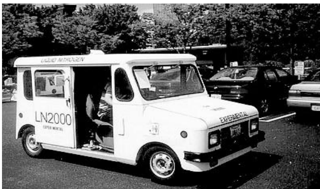
Figure 5 – LN2000 – experimental model of cryomobile operating on liquid nitrogen
