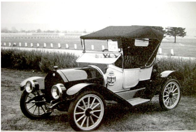
Figure 4 – “Little” – cryomobile working on liquid air (1914)
