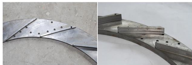
Figure 13 – Channel diffuser and holes for measuring static and total pressures
