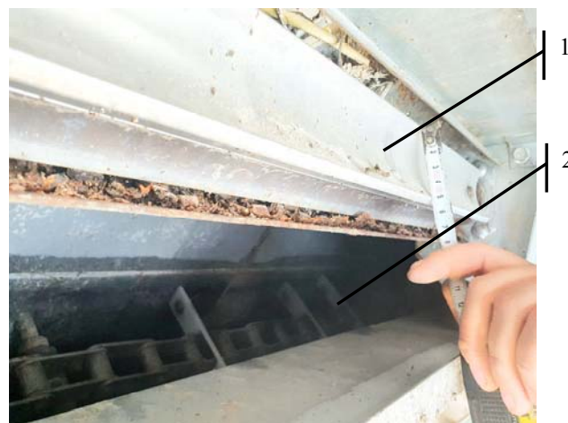
Fig. 4. Mechanism of grain unloading: 1-volume grain unloader, 2-scraper conveyor
