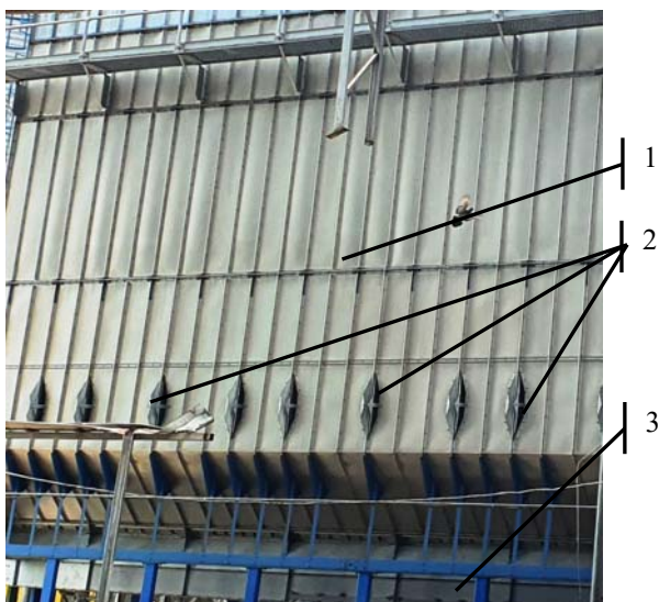
Fig. 3. Aerodynamic devices for control of heat recovery processes: 1 – cooling chamber, 2 – aerodynamic devices, 3 – mechanisms of grain unloading
