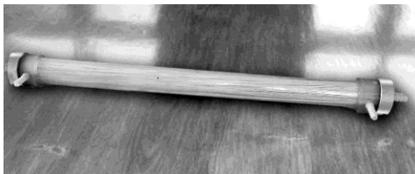
Fig. 2. The hollow-fiber membrane within module AR-1 (Mytishchi, Russia)
