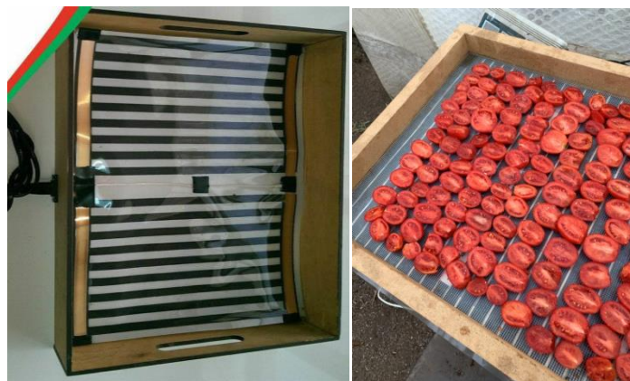
Fig. 1. Dryer tray with infrared film and prepared for drying raw materials
