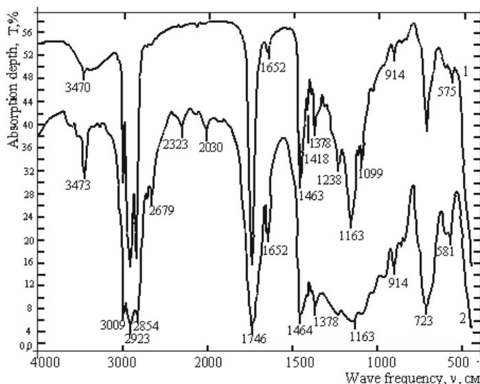
Fig. 2. IR spectra: 1 – sunflower oil, refined and deodorized (reference sample)
