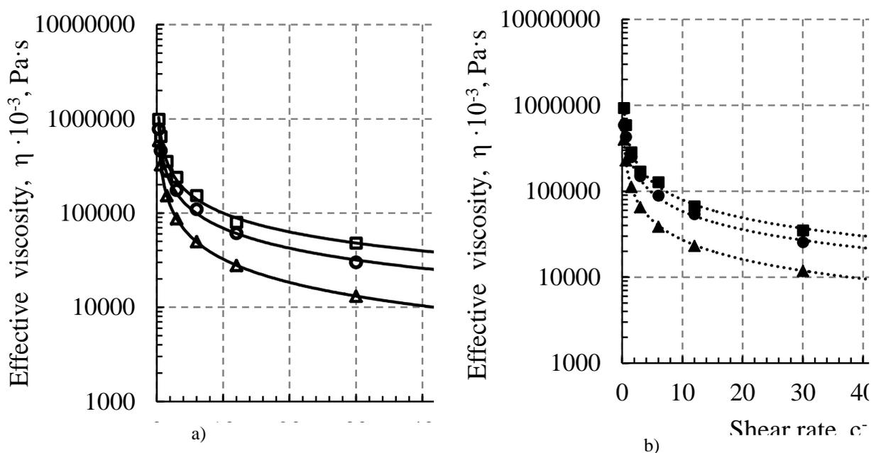
Fig. 4. Effective viscosity of emulsion-type sauces in a straight line (a) and in reverse (b)
