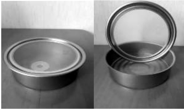
Fig. 1. Metal can with a lid made from the heat-resistant polymeric material PET/PE
