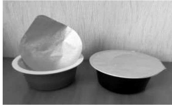
Fig. 2. Semi-rigid polymeric containers made from the multilayer barrier material PET/EVOH/ CPP, with aluminium foil covers coated with a thermoplastic
