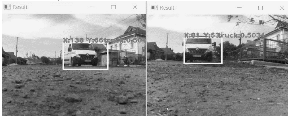
Fig. 7 – areas of recognized objects (a) in road traffic conditions
