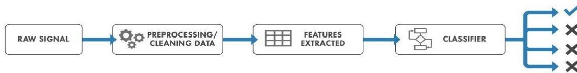
Fig. 8 – Schematic process for applying feature extraction to signals and time series data for a machine learning classifier
